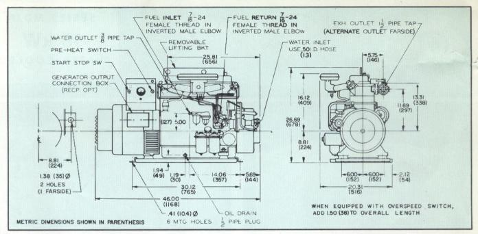
Add approx 1-in (25.4 mm) to overall dimensions for Heat Exchanger Cooled Models. Approx net weights: Raw Water Cooled 770-lb (349.27 kg). Heat Exchanger Cooled 790-lb (358.34 kg). Operation
